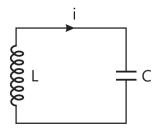
An LC circuit contains a 20 mH inductor and a 50  $\mu$ F capacitor with an initial charge of 10 mC. The resistance of the circuit is negligible. Let the instant of circuit is closed be t = 0.
